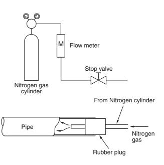
Fig. 6-5-1 Prevention of oxidation during brazing
